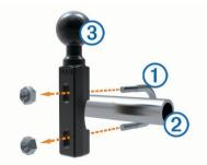
Tighten the nuts to secure the base.
