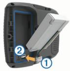
5 Close the battery cover and secure the battery cover D-ring.
